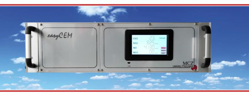
With the analyser EasyCEM gases can be measured such as CO, CO2, NO, SO2, SF6, THC with the NDIR method or with PID, as well as gases like NH3, HCI and CH4 with a TDLS (tunabel diode laser) By extending further modules with NDUV or electrochemical measuring principles, it is possible to measure gases like O2, O3 or NO2.
